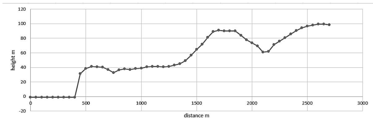
Figure 262: Land surface cross section plotted from Digital Elevation Model data
